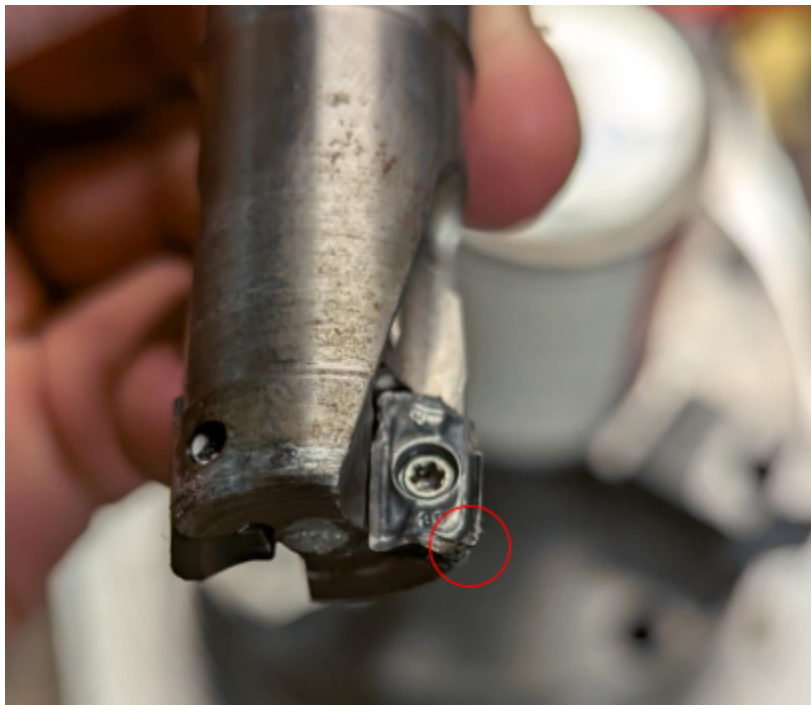
Figure 92: Damaged endmill insert, with damage circled in red
