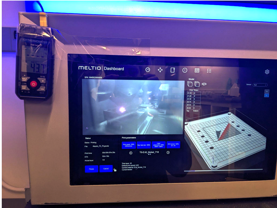
Figure 69: Meltio dashboard and thermocouple reading mid-print
