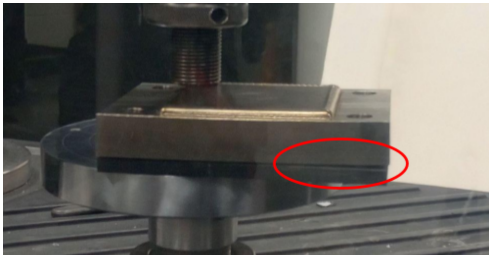
Figure 80: Corner forming gap between build plate and insulation due to warped build plate
