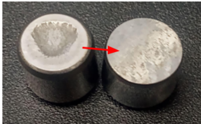
Figure 98: Dowel pin surface is grinded down for full contact as a forming tool
