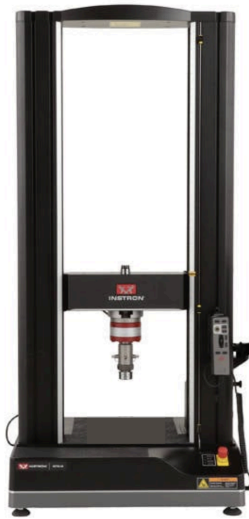
Figure 74: Instron Universal Testing Machine
